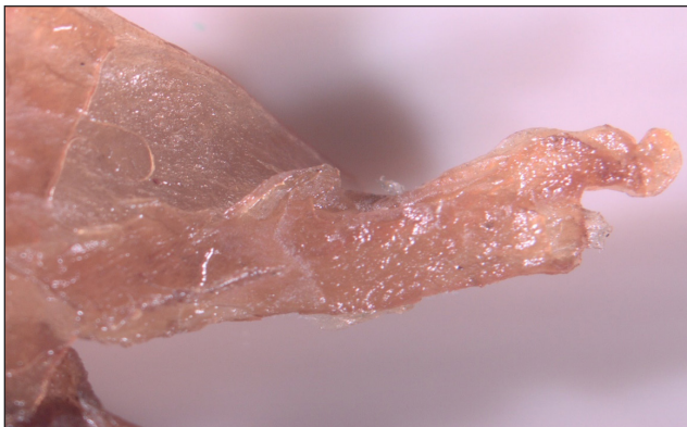
11. Gelatinous deposition found during the cleaning of a whitewater chest.
