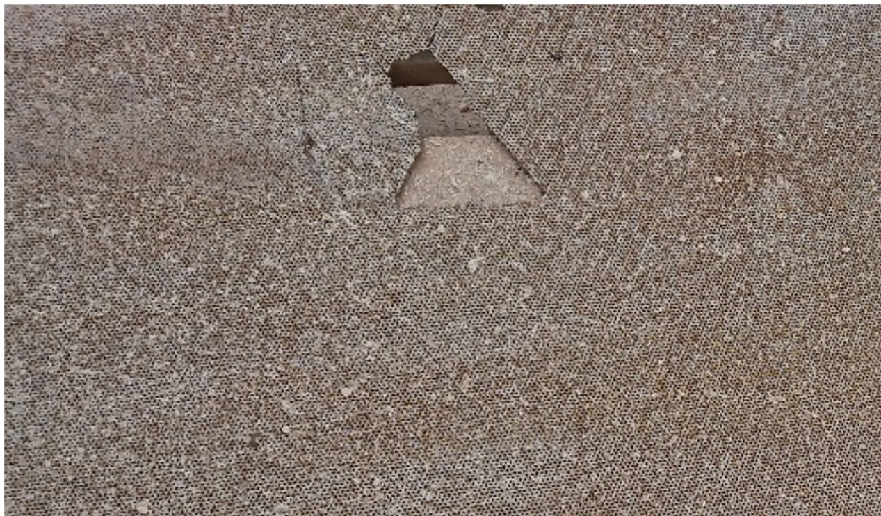
8. Detail from a screen plate in a hammer mill where the screen has a tear from a dislodged hammer.
