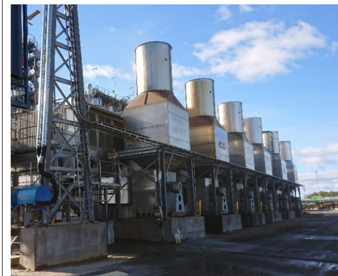
1. Belt dryer for sawdust (left) and storage silo (right) at the Värö mill in Sweden.
