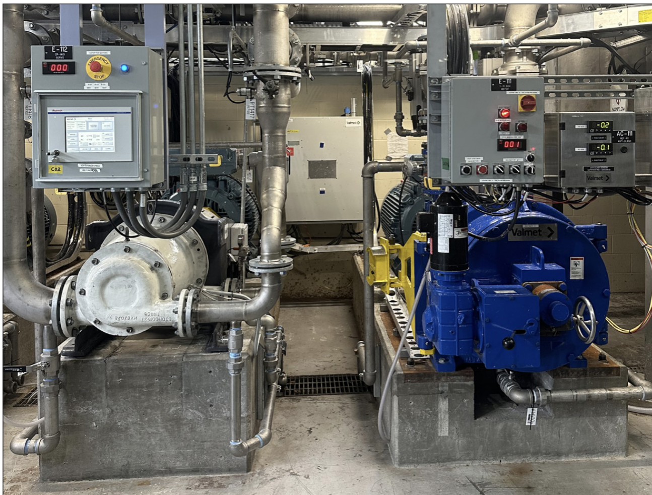
2. Valmet Optifiner PR01 conical refiner model (left) and DD6700 double disk refiner model (right). Photo courtesy University of Maine Process Development Center.
